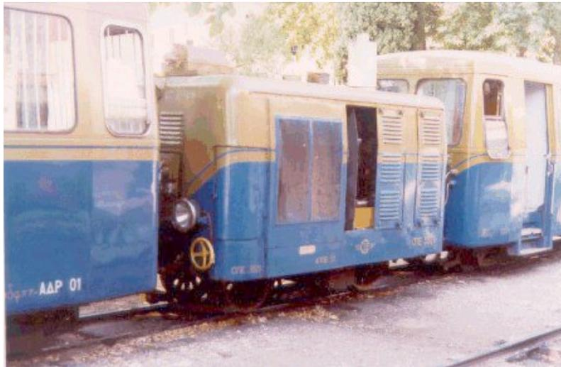
*The Diesel Electric DMU-2 3001, has a car between the two coaches which holds the diesel motor and the generator. This car is shown in the picture. The electric motors are located in the driving motor coach.*
