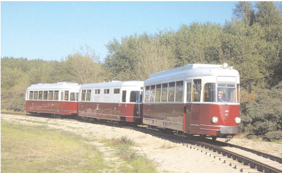
The photograph above shows the general arrangement of the set in use on the Zillertalbahn. The two ex DB trams are little modified apart from the provision of a power bus line in replacement for the pantograph. The home-built generator trailer is a remarkably good visual match; it runs on bogies recovered from a scrapped carriage.
