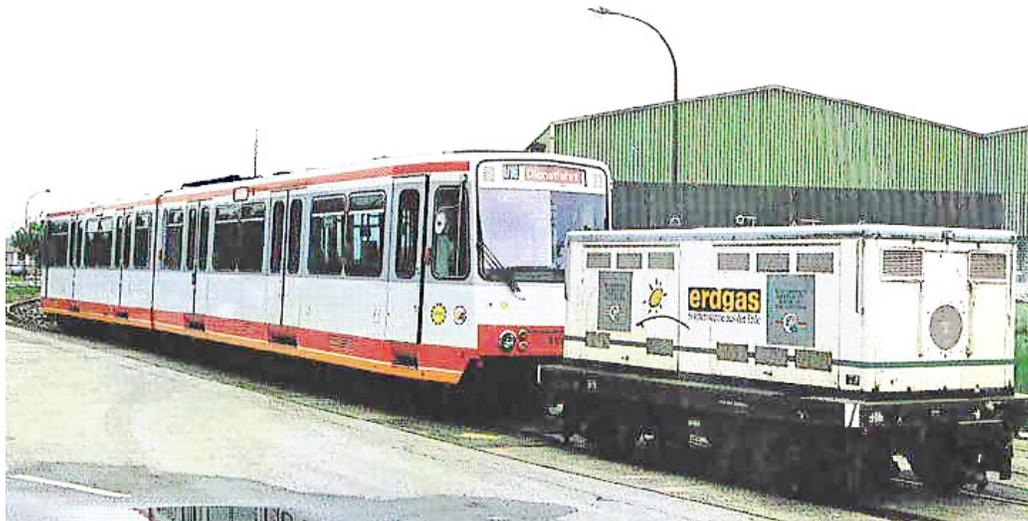
Experimental operation of a standard Stadtbahn car in Essen coupled to a natural gas – powered generator trailer. The unit was used to provide demonstration runs in 1999 as part of plans to bring a non-electrified industrial railway back into service as a light railway
